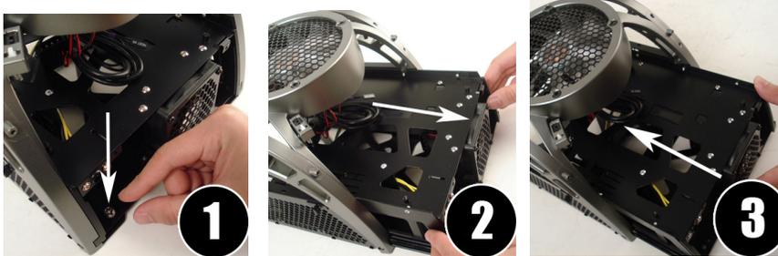
1. With the rear of the case facing you, remove the thumbscrew at the left side of the Component Tray.
