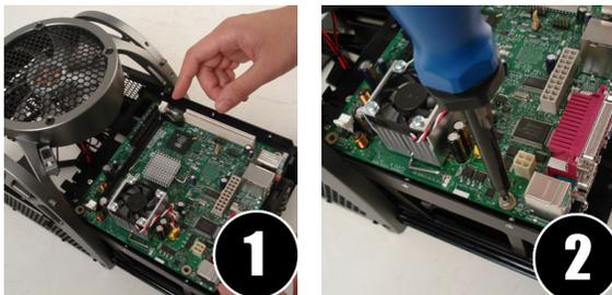
Slide out the Component Tray from the Frame as detailed in section 2.1.
