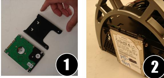
1. Align your 2.5" device with the included 2.5" device mounting plates and secure them together with the included screws.
