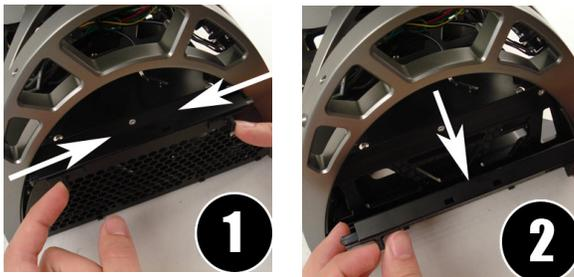
1. Locate and simultaneously press inward the two tabs on the left and right of the screen panel.
