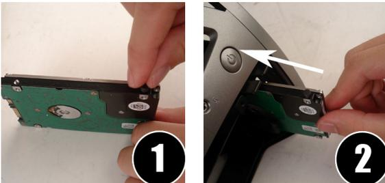
1. In your tool bag, find one of the black screws and attach one to your 2.5" device at the front screw holes.
